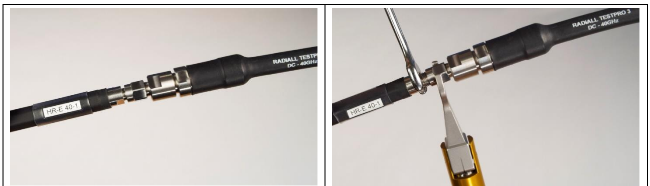
Figure 6: Connecting an RF cable to the HR probe
